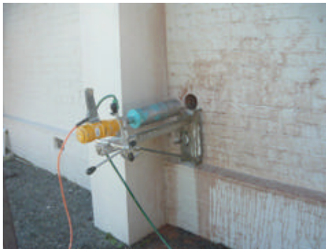
Core testing of brickwork – Auditorium wall, west face
